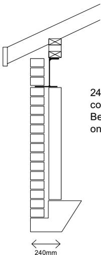
240mm brick veneer construction Shelf Beam sits generally on 89 x 89 SHS.
