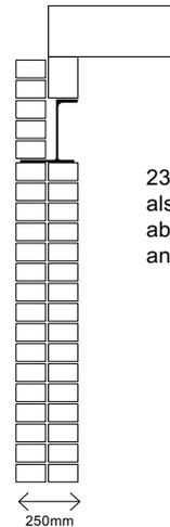
230mm solid brick (garage type) also allows for either jack stud wall above or stub column supporting another structural member.
